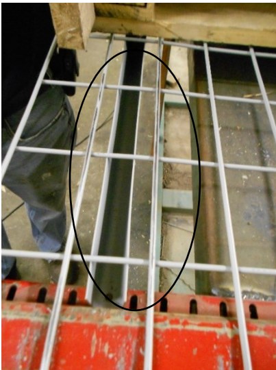
PAINTED DECK (Wear Visible at Wire Surface)
