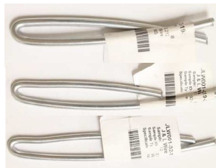
ZINC-COATED No Peeling Observed PASSED Bend Test
