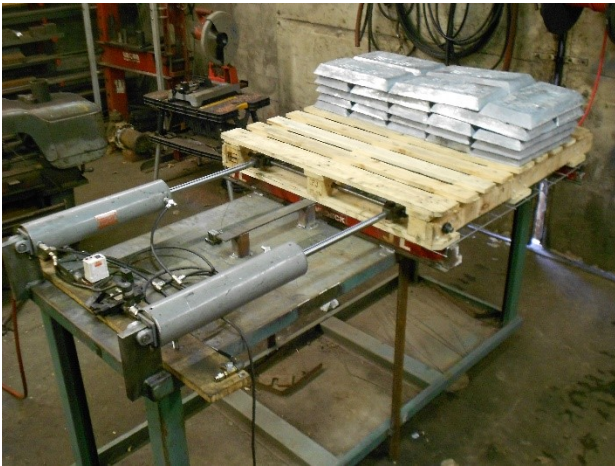
TEST APPARATUS (Hydraulic Cylinders, Pallet Weighted with Zinc)
